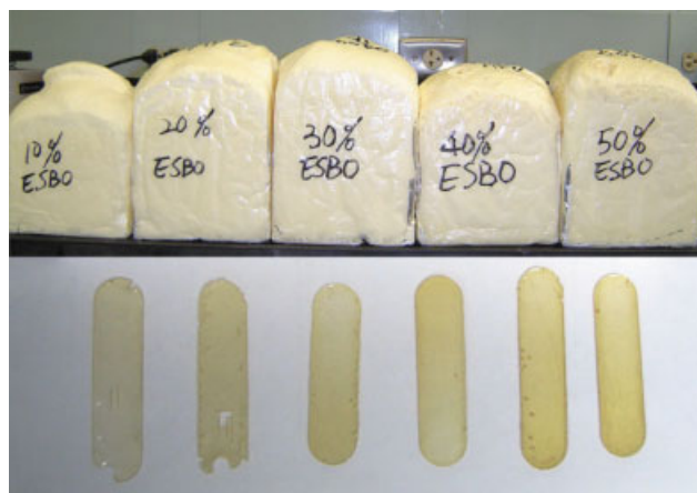
Figure 1 Water-blown flexible polyurethane foams and plastic films. The upper image shows flexible water-blown polyurethane foams with 10 to 50% ESBO. The lower image shows polyurethane plastic films with 0 to 50% ESBO from left to right. [Color figure can be viewed in the online issue, which is available at www.interscience.wiley.com .]
